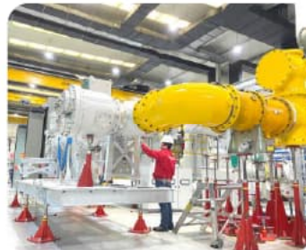
Testing of GIS modules and testing of the solution over the SKID to avoid part of on-site testing
